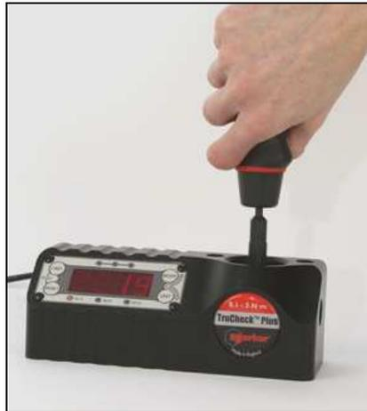
Norbar 0.1-3 N·m. TruCheck™ Plus Torque Screwdriver Tester
