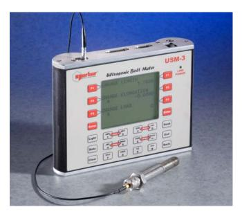
Norbar's portable USM-3 ultrasonic bolt meter measures the elongation and load in threaded fasteners, invaluable when the exact measure of fastener tension is essential for the integrity of a mechanical joint, such as applications in the aerospace industry or the Bloodhound SSC Project.
