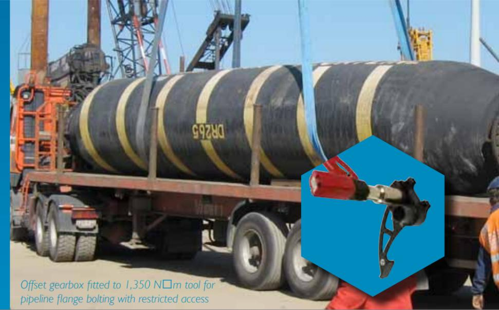
Offset gearbox fitted to 1,350 N·m tool for pipeline flange bolting with restricted access
