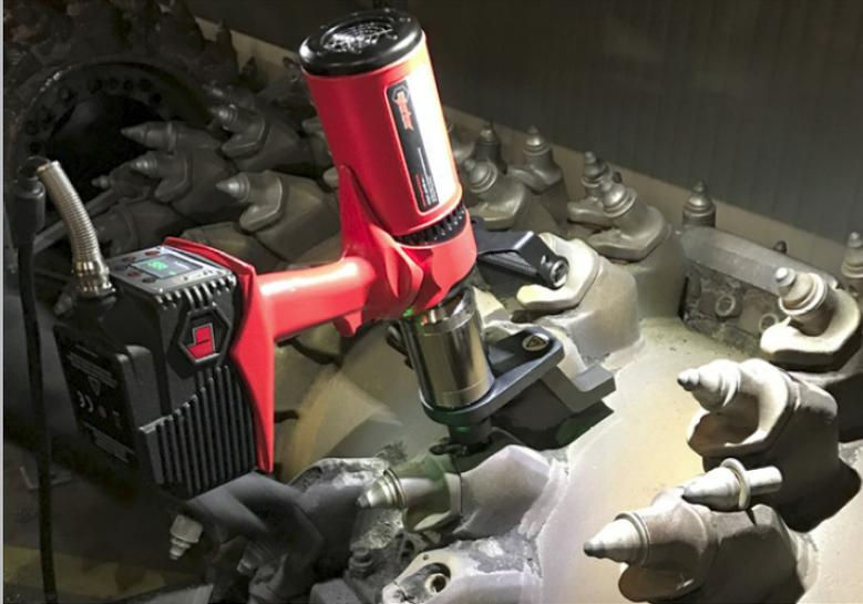
**Overview:** The basic components of a milling machine are a cutting drum to mill the existing pavement, a vacuum to collect the milled particles and a conveyance system to transport the milled particles to a dump truck for hauling. The cutting teeth shown in the image above are bolted to a roller assembly designed to penetrate a road surface.
