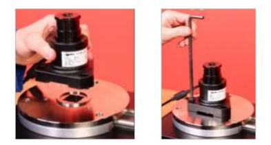
FIGURE 14 - Fitting an FMT Transducer
