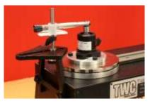
FIGURE 30 - Attaching FMT 2 to FMT 25 Adaptor Kit
