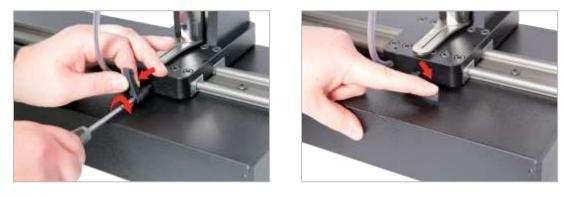
FIGURE 13 - Adjusting and Setting the Locking Lever
