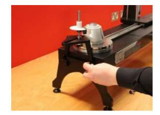
FIGURE 28 - Attaching Short Length Reaction Plate
