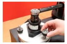
FIGURE 31 - Attaching FMT Quick Release Kit
