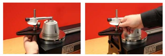
FIGURE 29 - Adjusting the Short Length Reaction Plates Reaction Point
