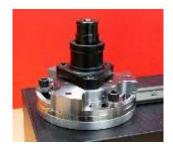
FIGURE 32 - Attaching TWC Angle Offset Plate
