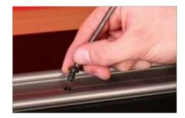
FIGURE 21 - Removing Button Head Cap Screw
