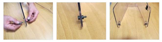
FIGURE 6 - Pairing the Neoprene Washers with Shoulder Bolts
