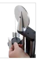
FIGURE 17 – Adding Weights to the Counterbalance Reaction Assembly
