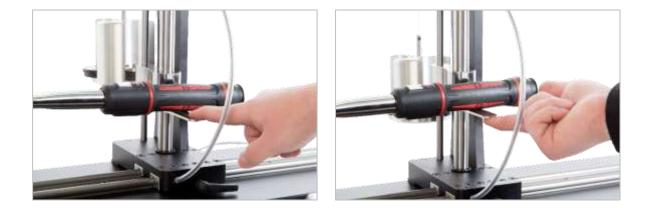
FIGURE 18 – Ensuring the Torque Wrench is in a Horizontal Position
