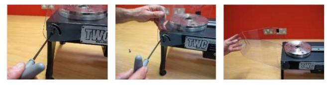
FIGURE 7 - Fitting the Guard
