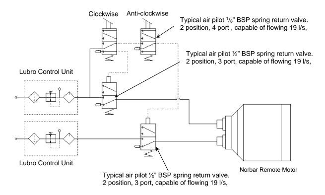
FIGURE 7 - Example of Pneumatic Circuit
