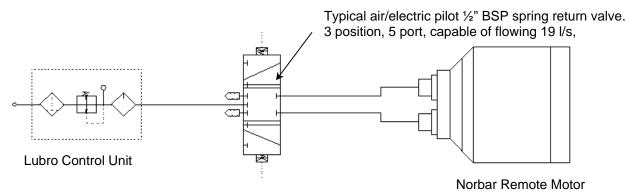
FIGURE 8 - Example of Pneumatic Circuit
