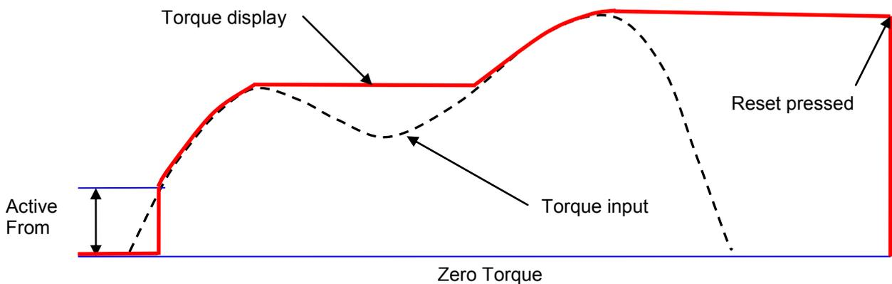
When Torque is applied, the NorTronic® will track the torque input until it has exceeded the **Active From** setting (See page 19) and then enters into peak mode for Torque & Angle.
