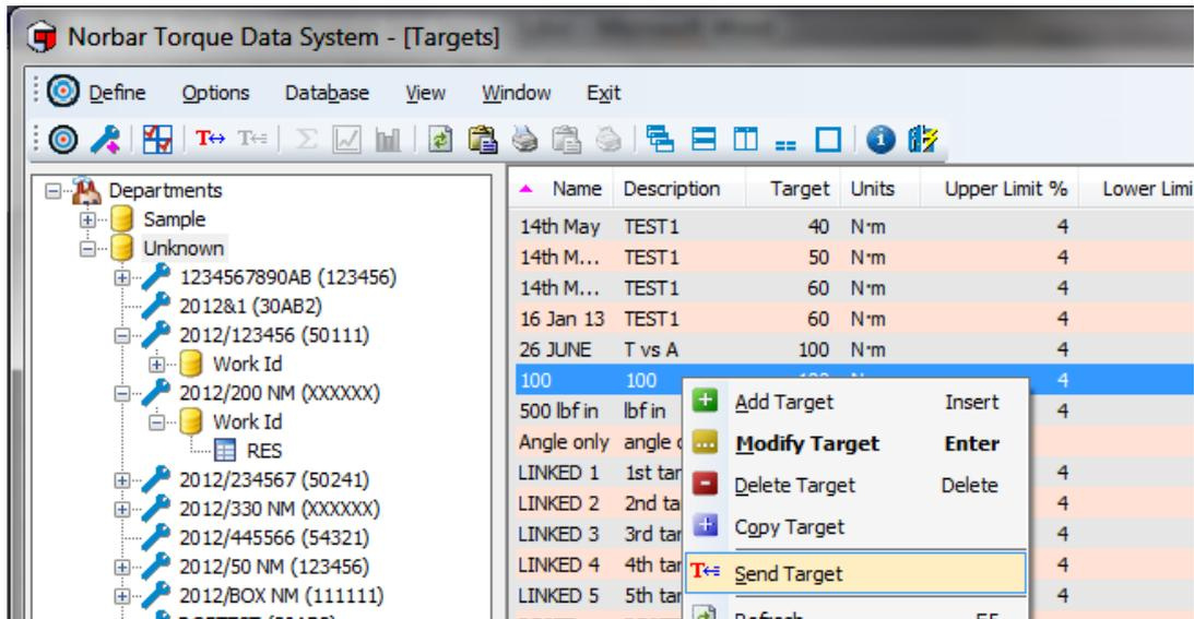
The **Target** can be changed on the tool unless the **“Locked”** option has been **ticked** in **“Set Tool Options”** and **downloaded** to the NorTronic<sup>®</sup> by clicking the **Update** button on **“Set Tool Options”** as shown below. (See page 16 for more information on **“Set Tool Options”**)
