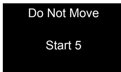
5 second countdown to the Gyroscope drift calculation.
