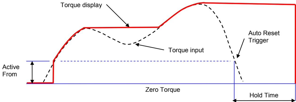
When Torque is applied, the NorTronic® will track the torque input until it has exceeded the **Active From** setting (See page 19) and then enters into peak mode for both Torque & Angle.
