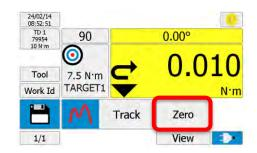
TIP: If the displayed reading does not zero the transducer may be overstrained. Contact a Norbar approved distributor for further advice.
