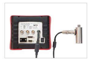
3. Connect up to 4 transducers to transducer connectors TD1, TD2, TD3 & TD4.
