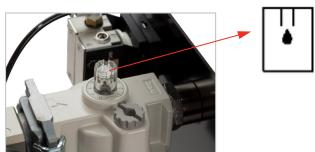
FIGURE 5 - Lubricator Flow
