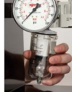
FIGURE 9 - Replacing the Filter Element
