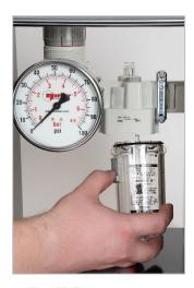
FIGURE 6 – Lubricator Bowl Replacement
