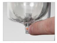
FIGURE 7 – Draining Condensate
