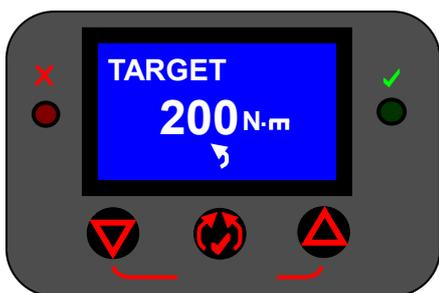
FIGURA 19 – Target torque
