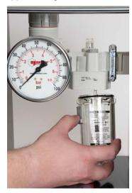
FIGURE 4 – Lubricator Bowl Replacement
