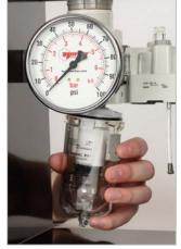
FIGURE 7 - Replacing the Filter Element
