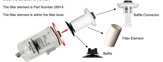
FIGURE 6 - Filter Bowl Components
