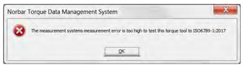
Check the measurement device and transducer uncertainty values are correct.
