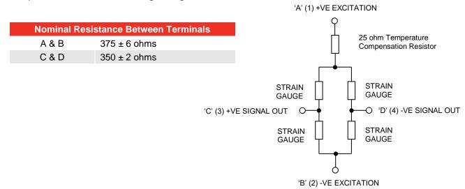
NOTE: ROTARY transducers do not have the 25 ohm Temperature Compensation Resistor fitted, so their A & B resistance is 350 ± 2 ohms.
