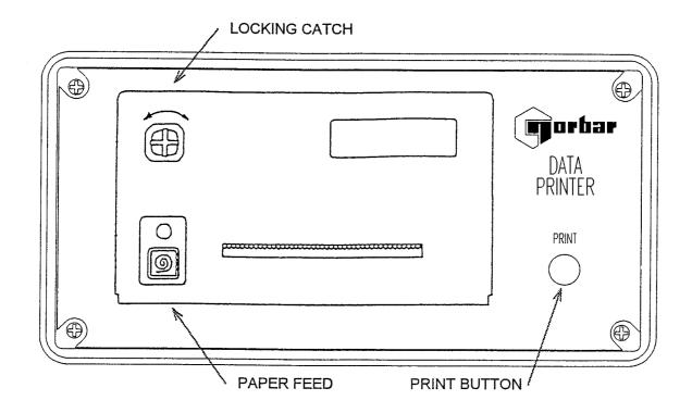
The Norbar Data Printer is a serial (RS232.C), dot matrix, impact ribbon printer that conforms to current EC Directives and Safety standards.
