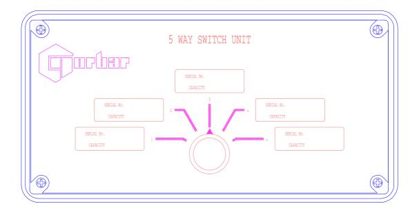
The Norbar 5 way switch unit conforms to the current EC Directives and safety standards. The unit enables any one of up to five Norbar transducers to be switched to the Norbar Electronic Transducer System (ETS), instrument.
