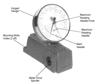
Select the appropriate splined adaptor to suit the square drive of the torque wrench to be tested. Insert this into the correct side of the meter drive spindle and fit the wrench into the adaptor ensuring that the wrench handle is approximately horizontal.
