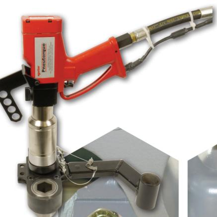
In this typical engineer to order application, the train operator was struggling to tighten the bolts pocketed into this casting. Norbar's solution was this special offset gearbox.
