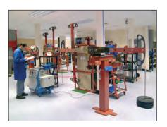
Production Line calibration equipment itself calibrated in Norbar's UKAS laboratory every four months.
