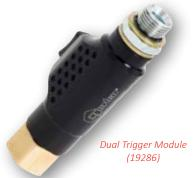
A secondary trigger for use with all PTS and PTM tools that easily attaches between the tool's air inlet port and hose. This requires the operator to use both hands to run the tool and so reduces the risk of hands getting trapped between the reaction bar and reaction point.
