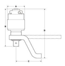
Alternative 350mm long, straight reaction plate; may be modified by customer to suit their applications. HT30 Part No. 16686 HT60 Part No. 16687
