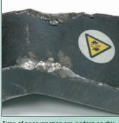
Signs of poor reaction are evident on this damaged foot. Reaction was taken at the wrong point on the foot and burring indicates that the foot was slipping off the reaction point.
