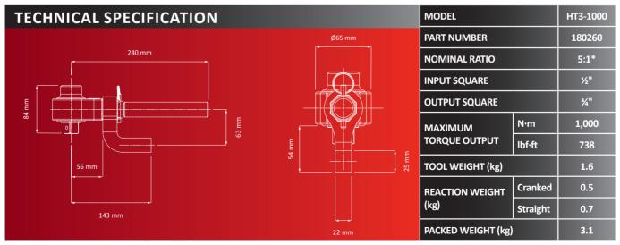
\*5:1 nominal torque multiplication reaction dependent. Ratio with cranked reaction is 4.8:1; with straight reaction being 4.9:1.
