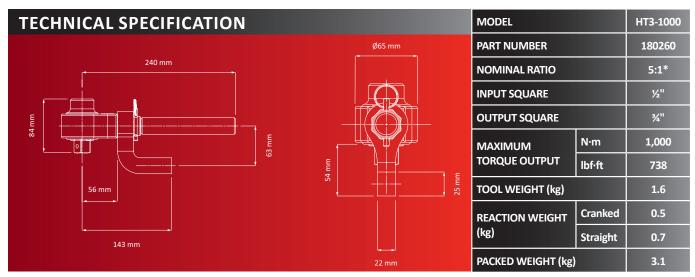
\*5:1 nominal torque multiplication reaction dependent. Ratio with cranked reaction is 4.8:1; with straight reaction being 4.9:1.
