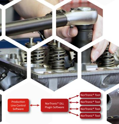
NorTronic<sup>®</sup> DLL (Dynamic Link Library) plugin enables NorTronic<sup>®</sup> 868 MHz and 915 MHz version tools to be interfaced to a customer's existing production line control software. DLL is not compatible with Bluetooth<sup>®</sup> versions. Contact Norbar for more details.
