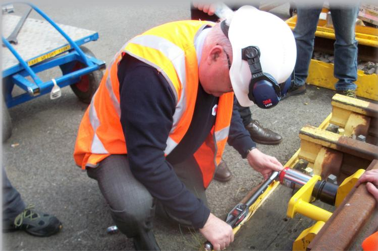
Codiun, a leading innovator, manufacturer and supplier of products to the rail industry recently met trackside with Norbar's own David Waters. They performed a series of tests using the Norbar designed NorTronic wrench and HT72 compact torque multiplier in conjunction with the Codiun designed Intelliclamp system.
