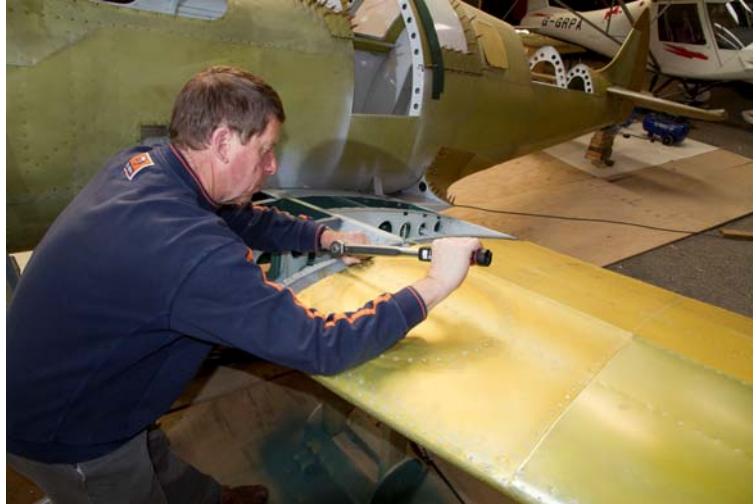
A Norbar Professional Model 200 torque wrench being used to assemble the wing onto a new MK26B Spitfire
