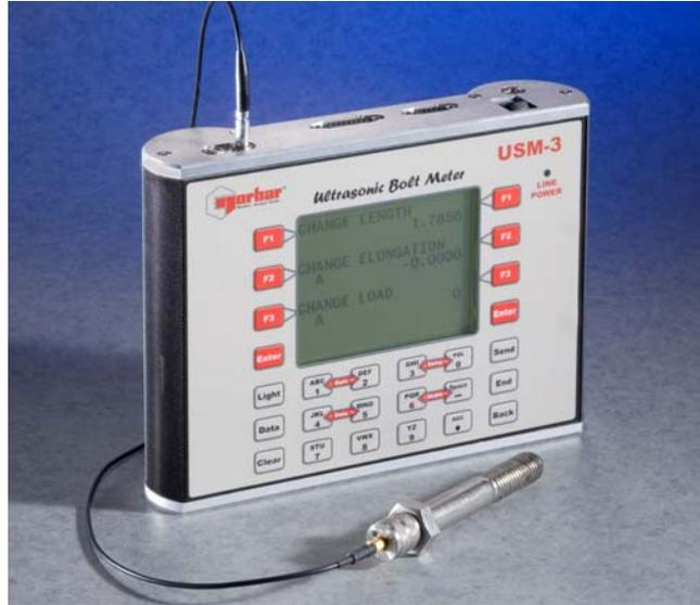
Norbar's portable USM-3 ultrasonic bolt meter measures the elongation and load in threaded fasteners, invaluable when the exact measure of fastener tension is essential for the integrity of a mechanical joint, such as applications in the aerospace industry or the Bloodhound SSC Project.
