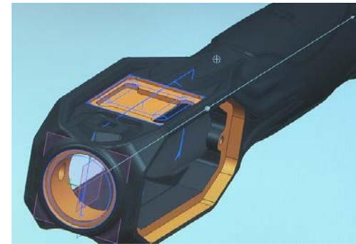
In terms of confidentiality, anything still within the research and development (R&D) department can be kept separate and, when communicating with customers, Norbar engineers use the Linked Exteriors feature of NX. This allows designers to put a skin on a gearbox assembly, for example, and then export it without the internals. The intellectual property in the gearbox design is thus protected when a model is sent to a customer for checking.
