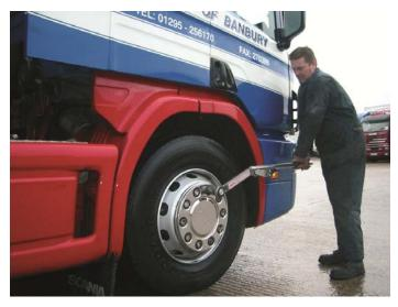
Norbar Industrial Torque Wrench being applied to Wheel Nut
