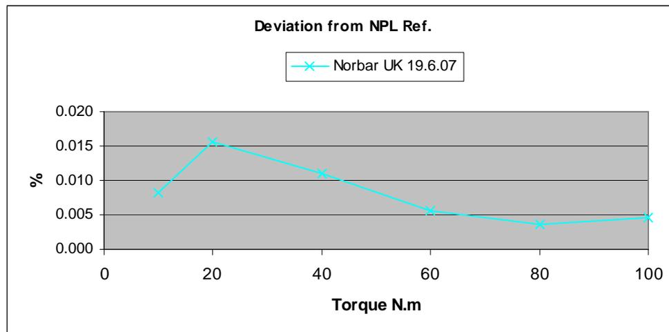
**Figure 3. deviation of a 100 N·m transducer from the NPL reference value.**
