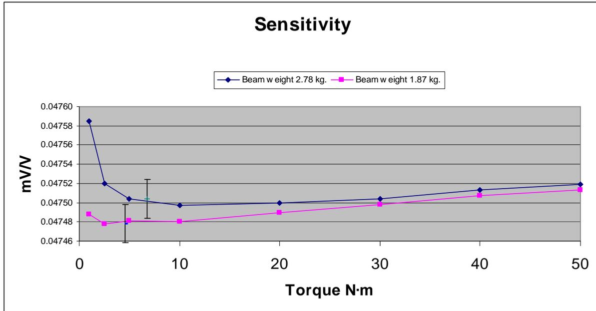
Figure 1. Sensitivity of a 50 N·m transducer calibrated with unsupported calibration beams.
