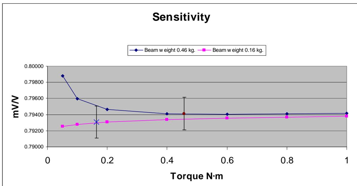
Figure 2. Sensitivity of a 1 N·m transducer calibrated with unsupported calibration beams.
