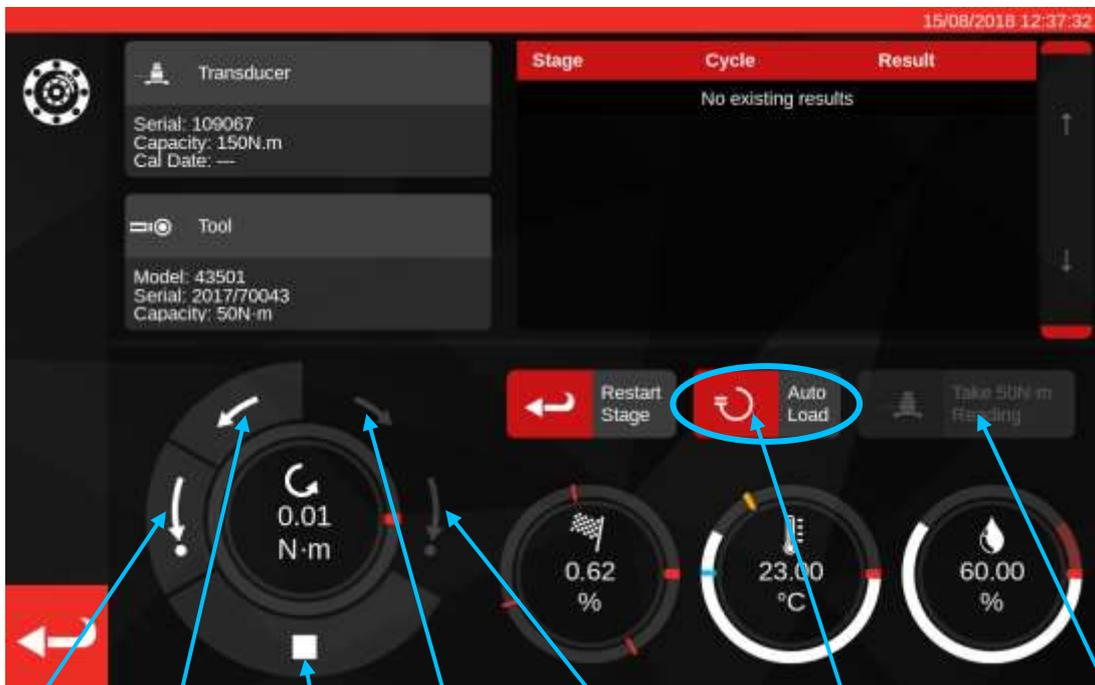
Home CCW    Nudge CCW    Stop    Nudge CW    Home CW    Load to nominal 80% of target torque    Take reading (capture value)
