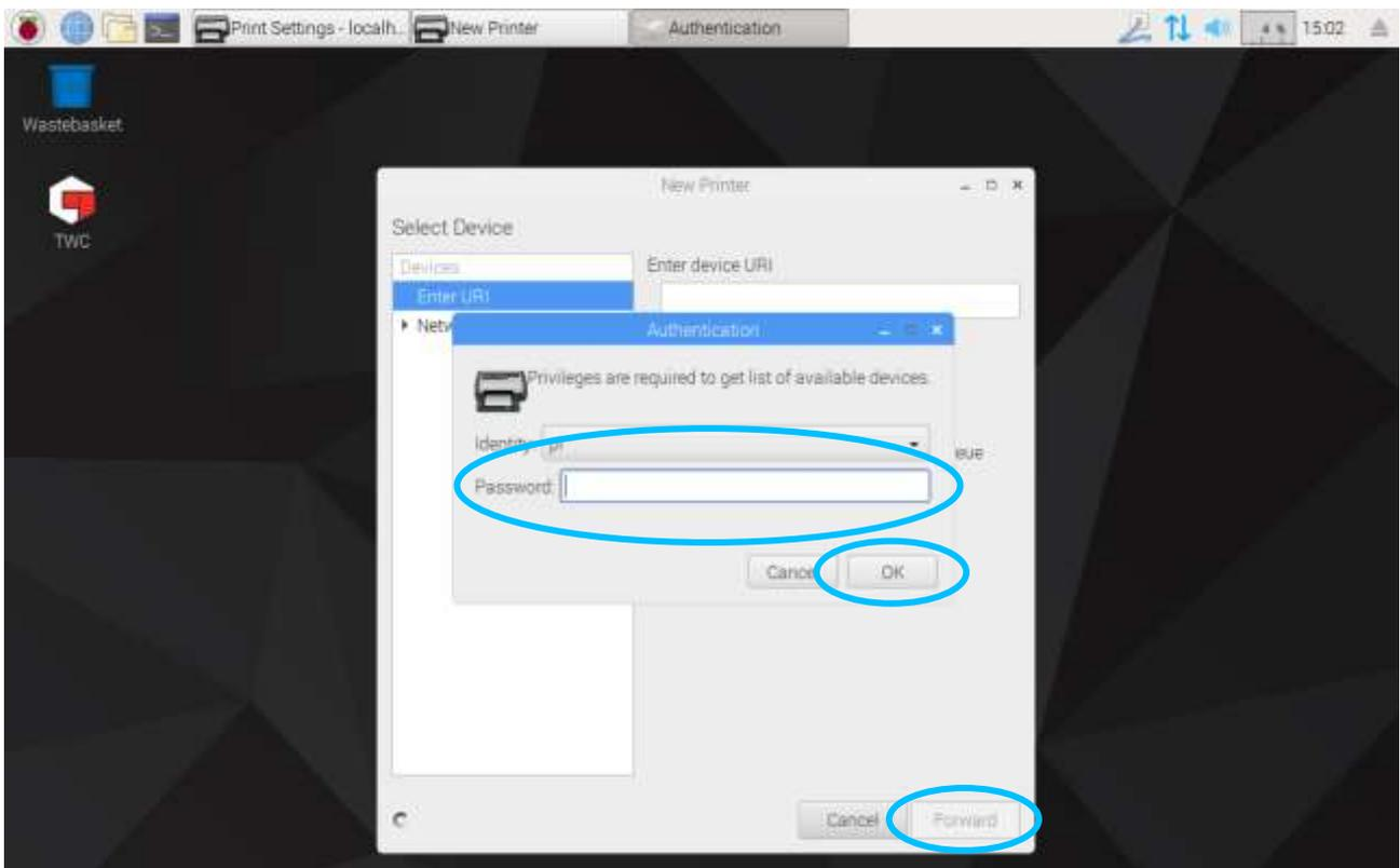
In the left-hand list will appear a USB-attached printer if currently connected. Beneath this, under the Network Printer drop-down menu, network printers will appear as and when the TWC finds them (this may take several seconds).
