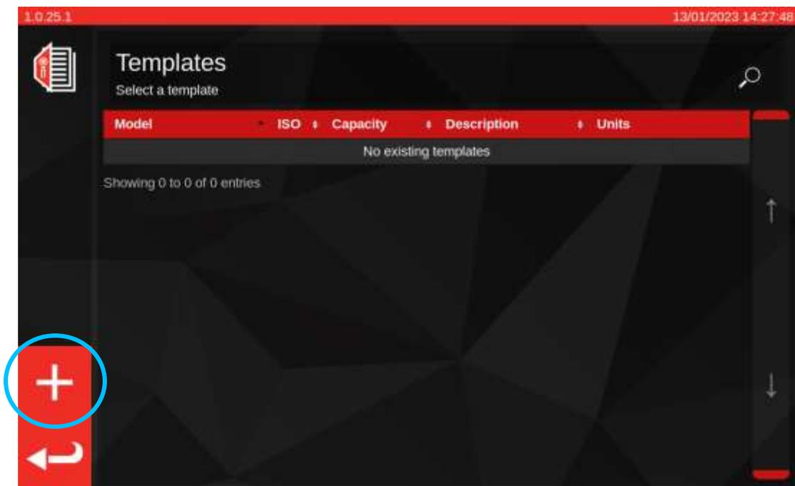
The Template Editor allows you to define all the parameters of a tool model which are necessary for the TWC to calibrate it properly.
