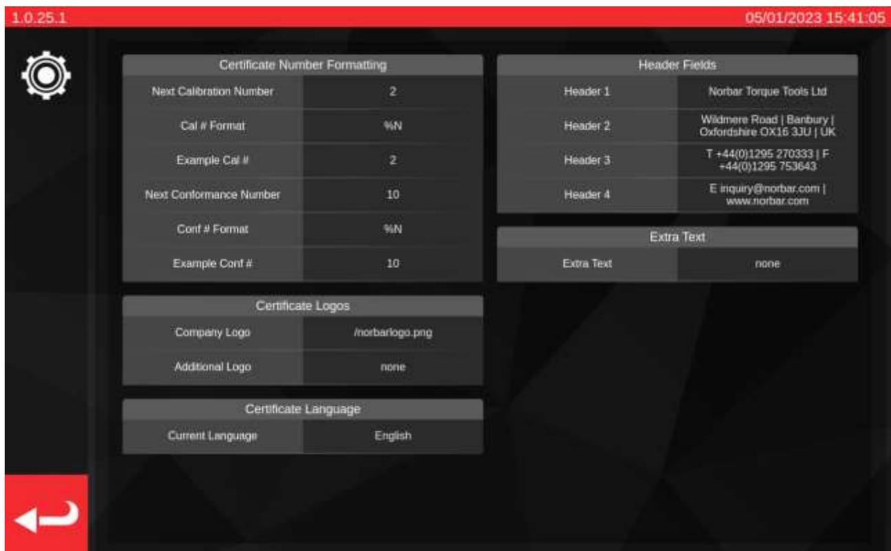
**Next Calibration / Next Conformance number:** for traceability, each calibration or conformance document is numbered, with the number increasing every time one is produced. You can set or change that number here for both types of document.
