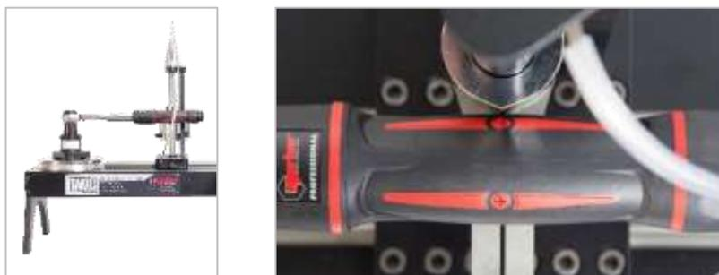
**FIGURE 16 – Locating a Torque Wrench**
