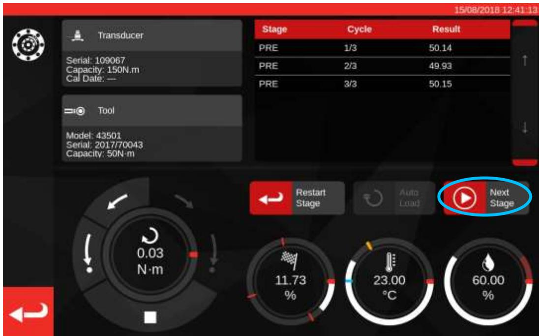
Once Preloading is complete, the 'Take Reading' button will change to 'Next Stage'. Press 'Next Stage' to advance to the next stage of the workflow.
