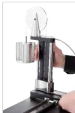
**FIGURE 12 – Sliding the Counterbalance Reaction Assembly onto the Reaction Rail**
