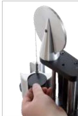
**FIGURE 17 – Adding Weights to the Counterbalance Reaction Assembly**
