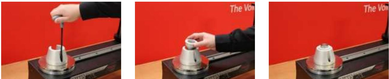
**FIGURE 27 – Fitting Static Transducer Support Kit**
