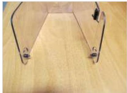
**FIGURE 6 –** Pairing the Neoprene Washers with Shoulder Bolts
