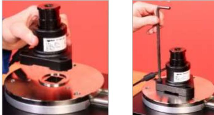
**FIGURE 14 – Fitting an FMT Transducer**
