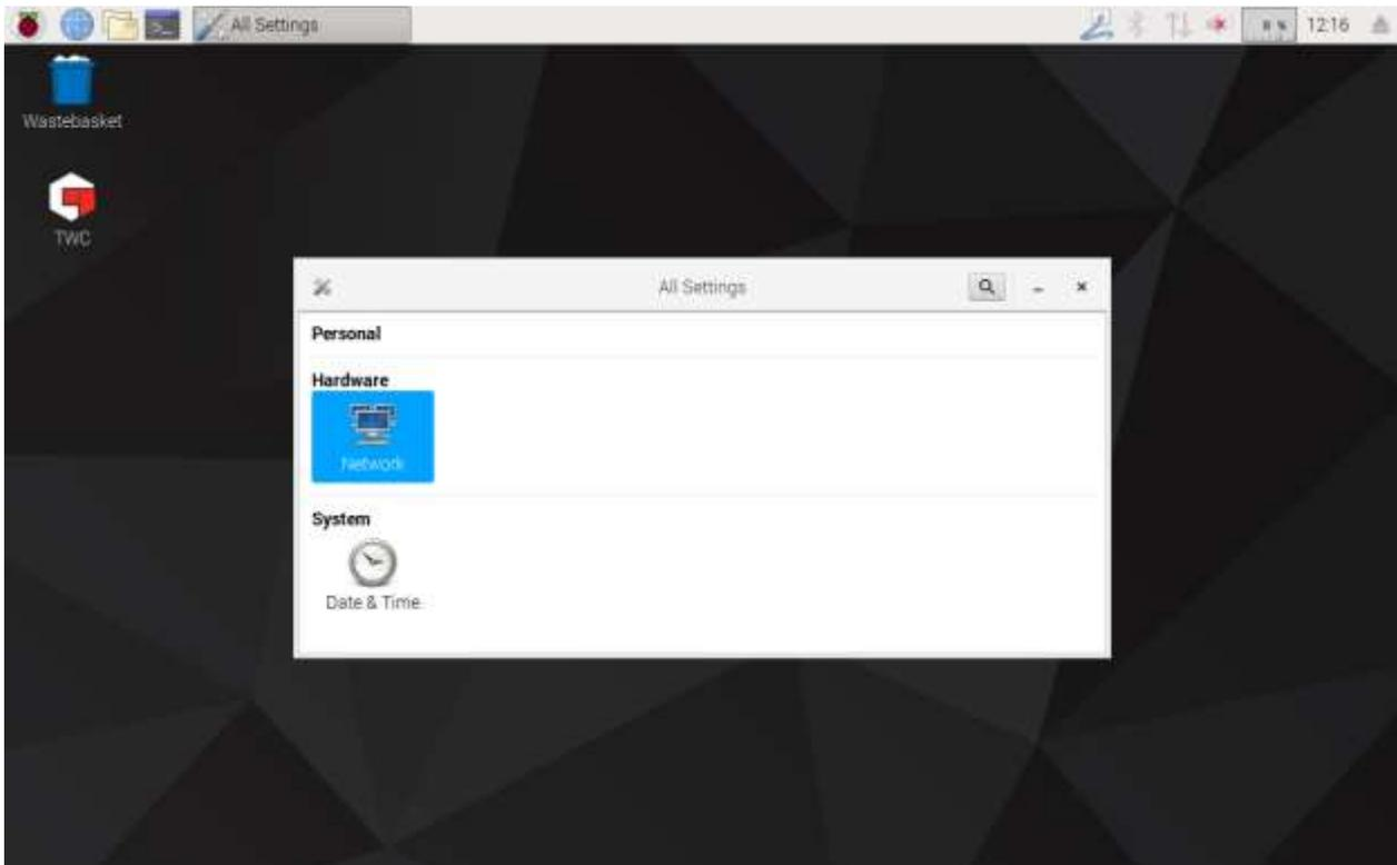
The panel will show the current network state. You should see something like the below if a network cable is connected. Ensure the Wired connection is selected, as shown here and press the settings icon in the bottom right to open the network settings panel.
