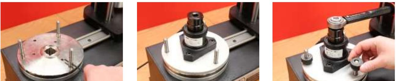
**FIGURE 31** – Attaching FMT Quick Release Kit
