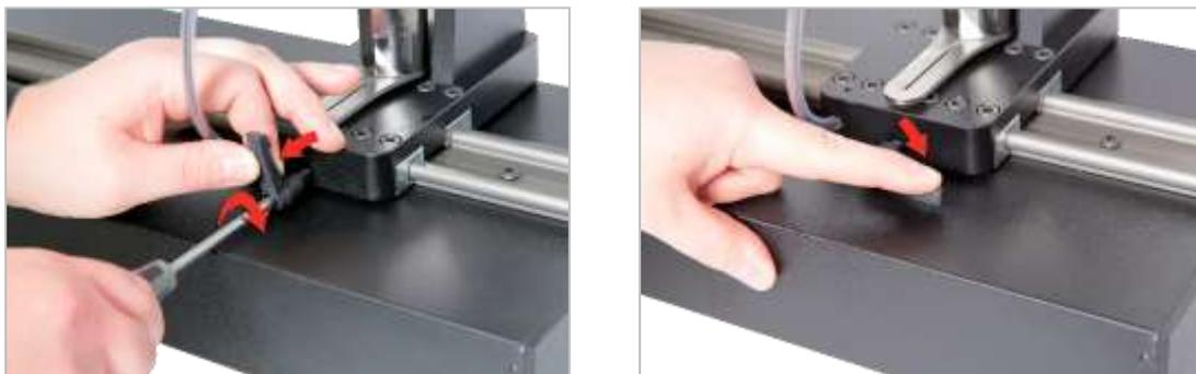
**FIGURE 13 – Adjusting and Setting the Locking Lever**
