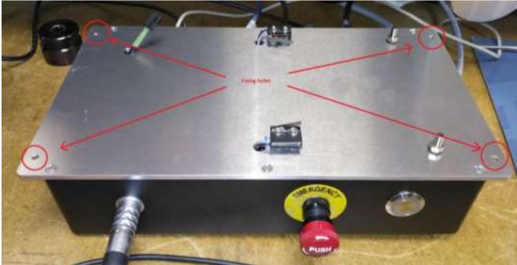
2. Next carefully lower the box. The connector of the guard sensor is inside the frame, to expose, gently ease out the cable.
