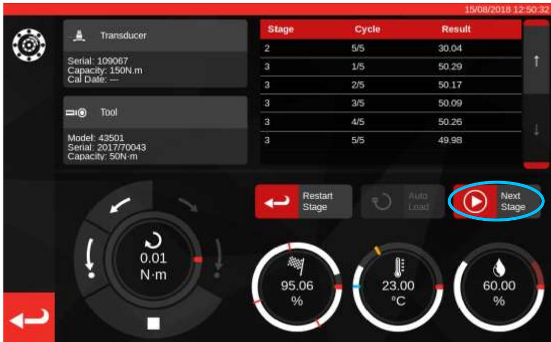
When the final stage is completed, press 'Next Stage' one final time to advance to the finish screen.
