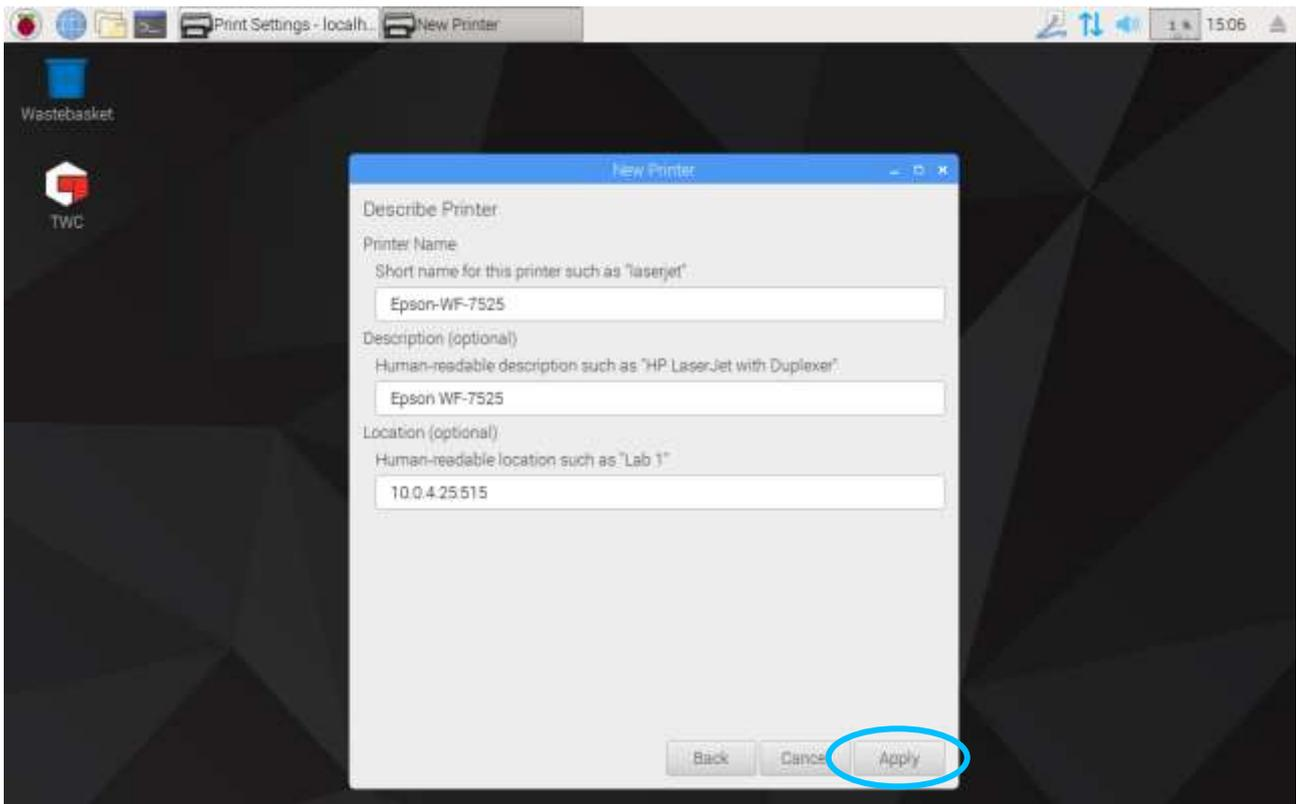
At this point the printer is added and you can print a test page. The printer will appear as an option when printing certificates or declarations of conformance from the TWC UI.
