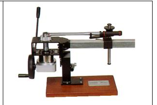
To change to the vertical position push the "ORIENTATION RELEASE HANDLE" (see drawing on page 3) to "RELEASE" position.
